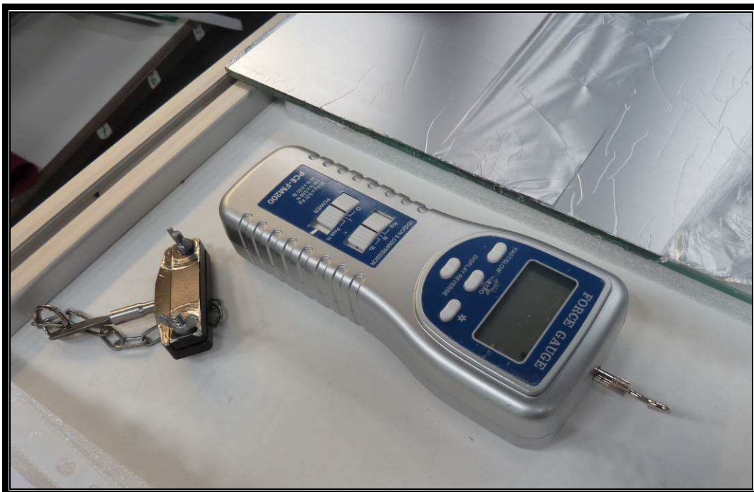
Picture 1: Hand force gauge and grip
