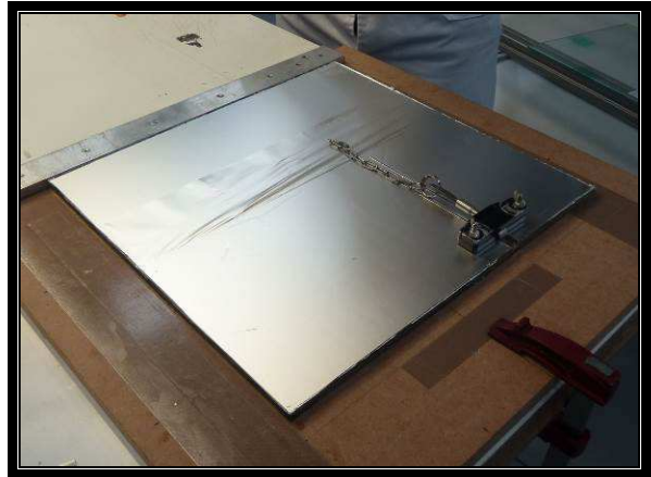
Picture 7: Grip fastened to the strip
