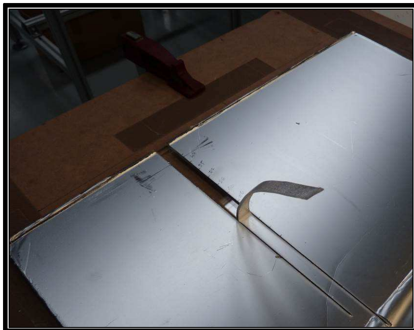
Picture 13: Final status of the polyvinyl butyral interlayer.
