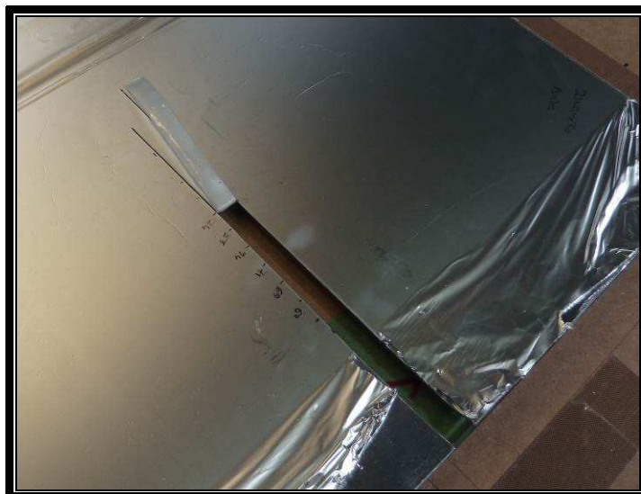
Picture 10: Final status of the upper pane of the ionoplast interlayer.
