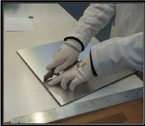
Picture 3: Cutting process of the 1 cm strip
