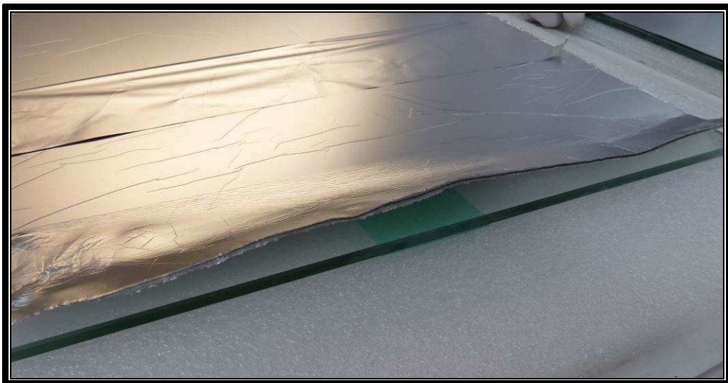
Picture 2: Edge of interlayer with aluminium film on both sides
