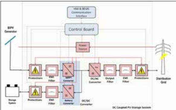
**Figure 5. (Above) Power Board of the SiC current source inverter designed (soft and hard) by CEA-LITEN-INES (width 390mm x depth 245mm). (Below) Block diagram of the 10 kW three-phase DC-coupled PV storage system developed by TECNALIA**
